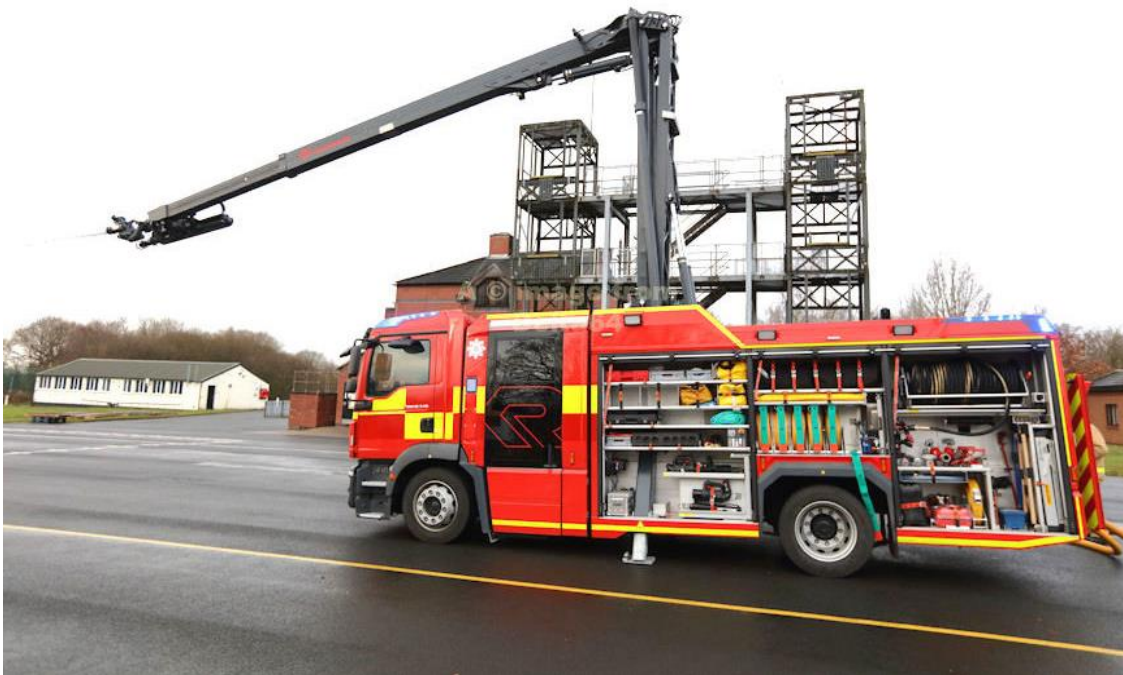
Figure 3 - Water Tower (Stinger) pumping appliance
